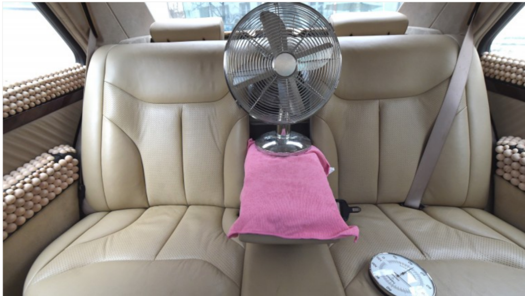
The hot air comes into the interior via a fan through a hole in the back seat (Photo: Ufuk Ucta)
